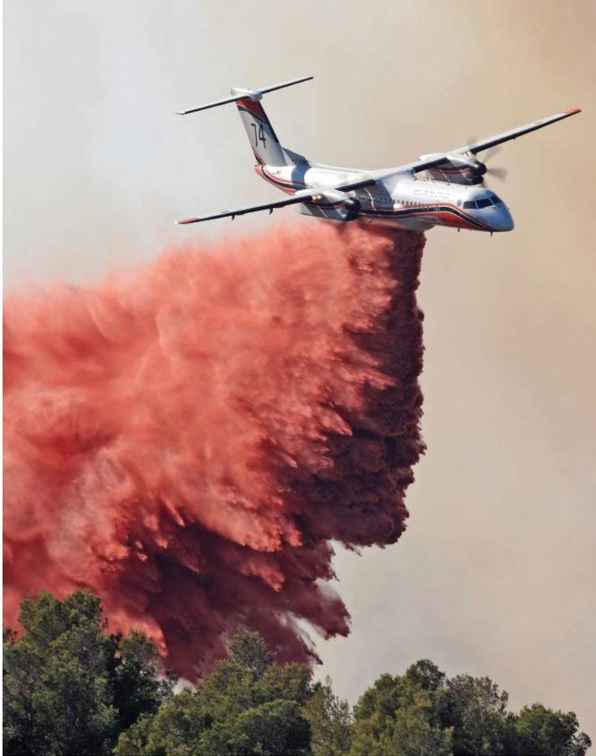
Engineers at Conair designed the Q400AT tank to deliver a 10,000-litre payload at any Interagency Airtanker Board coverage level.
