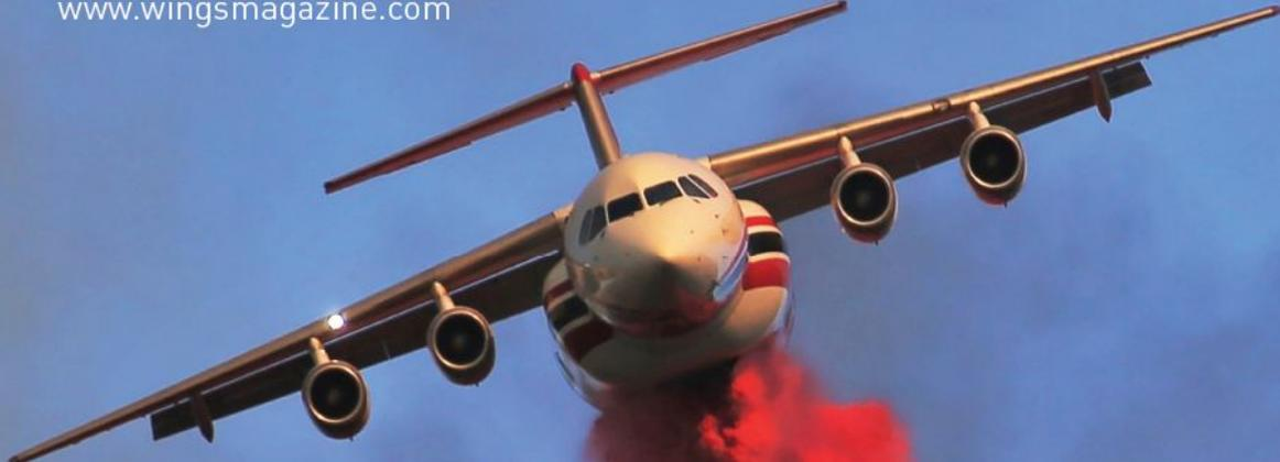
A Conair Avro RJ85 aircraft is shown from a low angle, flying towards the viewer. It is dropping a large, thick plume of red fire retardant from its cargo bay. The aircraft has a white fuselage with red and blue stripes on the nose and tail. The background is a clear blue sky.
